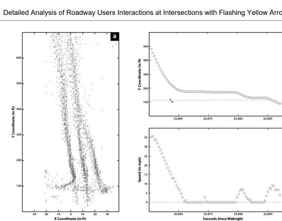
Figure 3.2 Visualization of Trajectory Dataset
