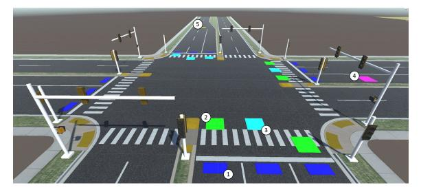
Figure 4.3 Sensors to Control Ambient Traffic
