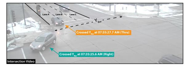
Figure 3.1 Intersection Characteristics and Information Logged for Vehicles from Video
